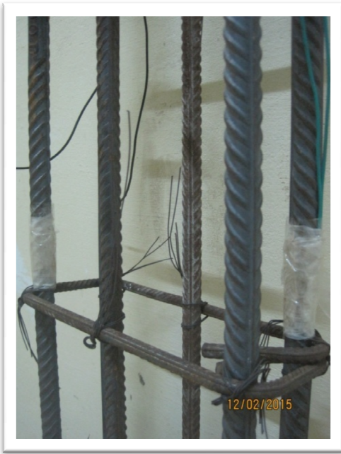
Fig. 3 Location of Strain gauge
